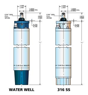
Note: 60 Hz - 3,450 RPM 50 Hz - 2,875 RPM
