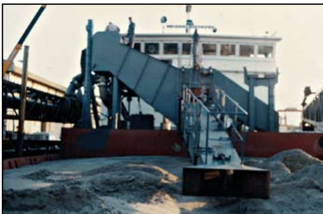
Model : DP 150 A. Application : Sand Collection from Sea View of Shooter Customer : Japan
