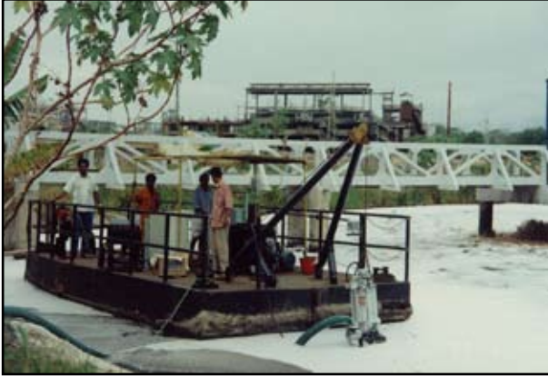
Model : DP 20 S on Pontoon Application : Effluents Lagoon De-silting Customer : SIV, India.
