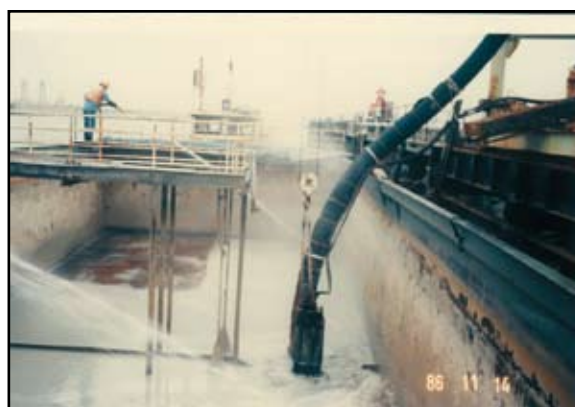
Model : Toyo Pump DP 30 B Application : Unloading of Silica from Barge. Customer : Glass Factory, Japan.
