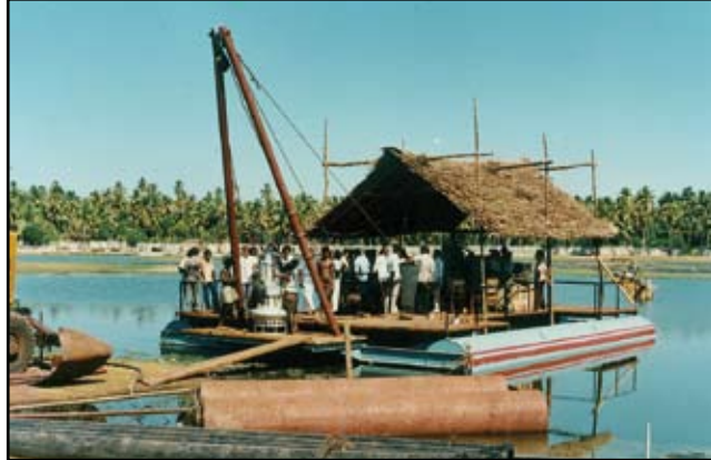
Model : DP 100 B on temporary Pontoon Application : For sand dredging Customer : Harbour Engg. Dept., Kerala, Neendakara Fishing Harbour
