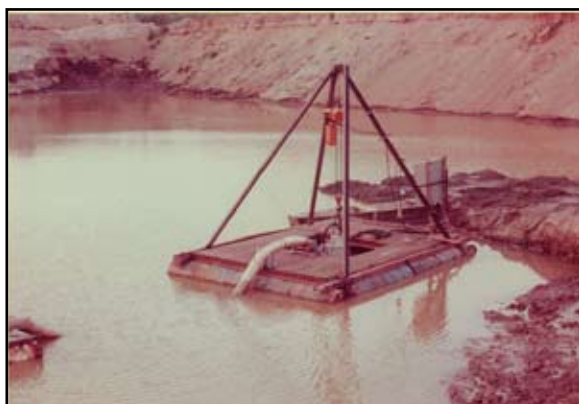
Model : DP 50 on Oil Drum Pontoon Application : Dredging Customer : USA
