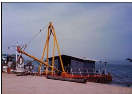
Model : Toyo Pump DP 100 B on Pontoon Application : Dredging in Fishing Harbour, Tadri. Customer : Karnataka Govt. / Indo Danish Fisheries Project
